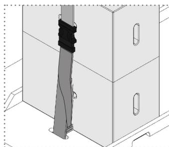
Stowage of X-belt in Xbrick grip hole or between X-belt and Xbrick
